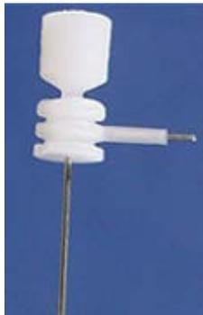
Has a plastic pedestal molded around an L-shaped stainless steel tube that extends below the pedestal and to the side to connect to the pump. A break-off segment fits in the MH-300 mounting holder for placement. After the Cerebond, dental cement or cyanoacrylate gel has set, the segment is cut off. The remaining pedestal is then covered with skin and sutured for a subcutaneous mounting. 3280P and 3300P have a 21 gauge side arm. 3220P has a 22 gauge side arm.
