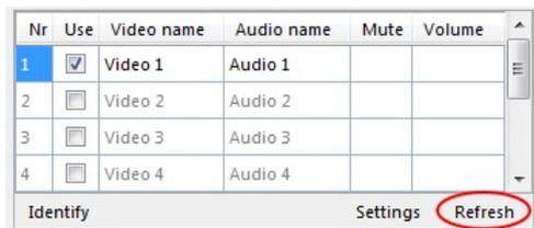
6. **Identify button** — To view which video number in the table corresponds with which camera source.
