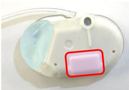
Magnet should be sterilized prior to use. Alternatively, use a sterile surgical drape or sterile plastic wrap around magnet to keep the pump sterile. Switch ON pumps sequentially, 5s per pump directly above magnetic switch. **Remove the magnet perpendicularly away from the top of the pump.** Keep the pumps in switching ON order by the UCD-X10R. As the pumps are switched ON, they will start to communicate with UCD-X10R.
