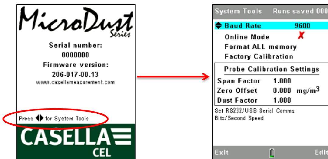
The **System Tools** screen should only be used for diagnostics or to configure the instrument for specialised applications. This screen allows you to do the following:-
