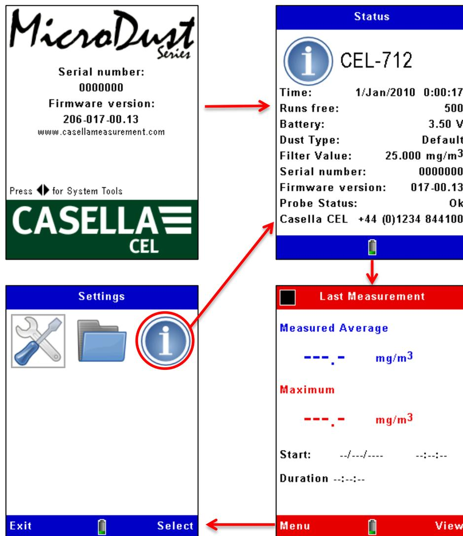
If the instrument has recorded a measurement Run since it was switched on, the measurement screen will show the average and maximum readings from that Run. Otherwise, the data fields will be null: - '---,-'.
