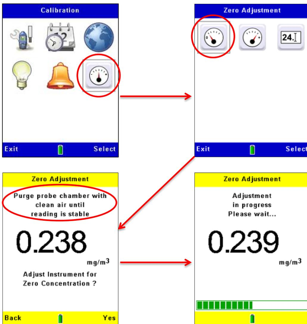
If the calibration fails, purge the probe with clean air for a longer period and then repeat the calibration procedure.
