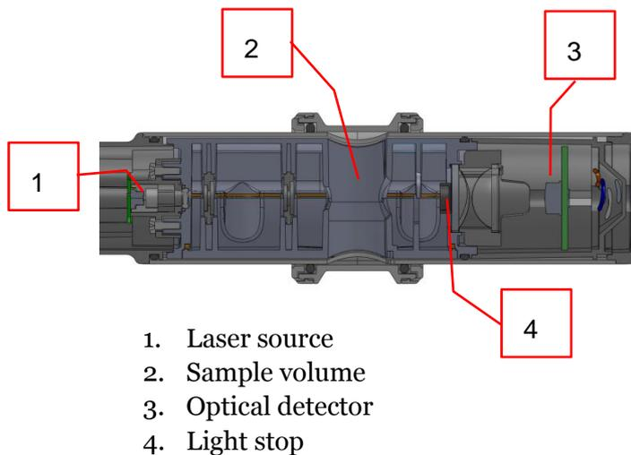
Under clean-air conditions, all light is prevented from following a direct route to reach the laser detector (3) by a light stop (4). When dust particles enter the sample volume (2), the beam of laser light is scattered within a narrow angle and some of it can reach the detector by indirect routes.
