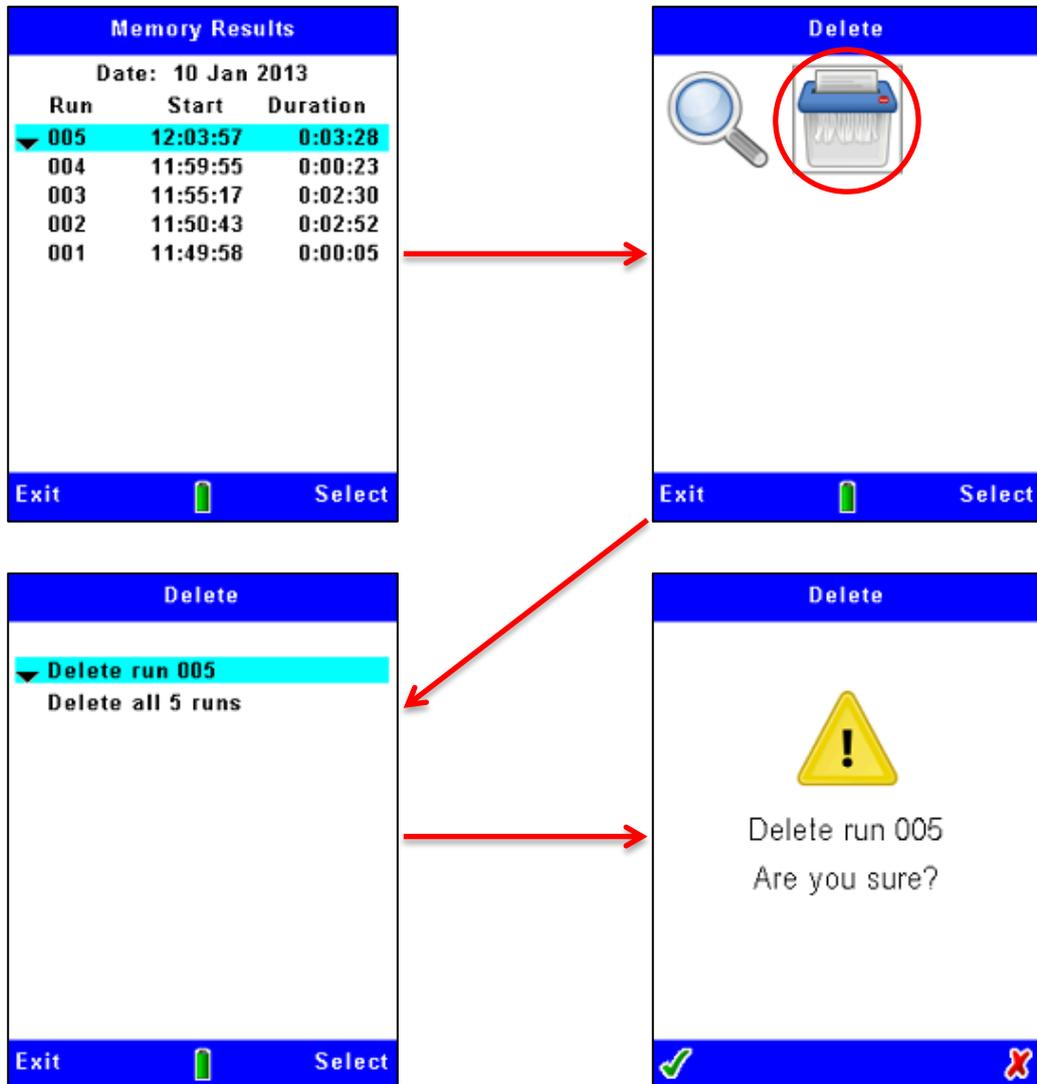
**Note:-** when you delete Runs from the instrument’s internal memory you cannot restore them again! Before deleting data files within the instrument, always use the Casella Insight Data Management Software application to safely transfer and save results to the PC.
