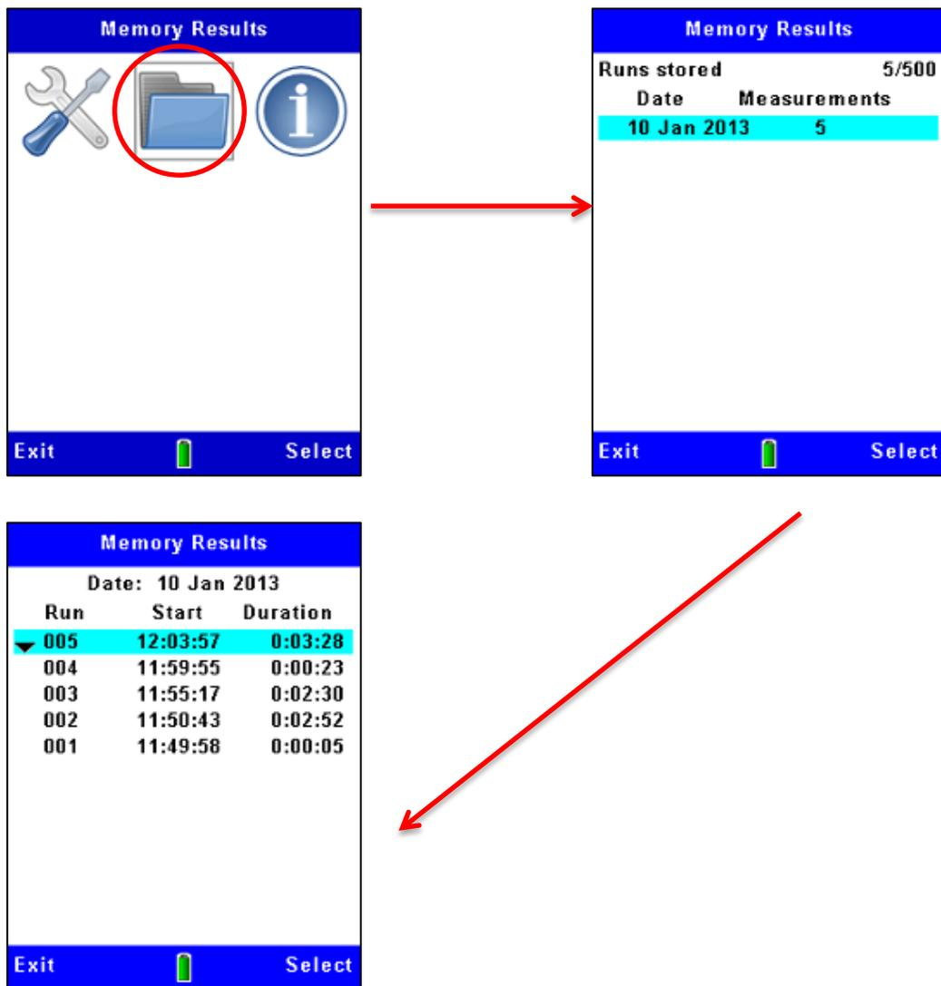
Use the up and down navigation keys ▲ ▼ to select one of the dates in the list, and press the Select soft key to show all the Runs recorded on that date. The Runs on each date are numbered sequentially beginning at Run 01. The earliest Run on a date is at the top of the list.
