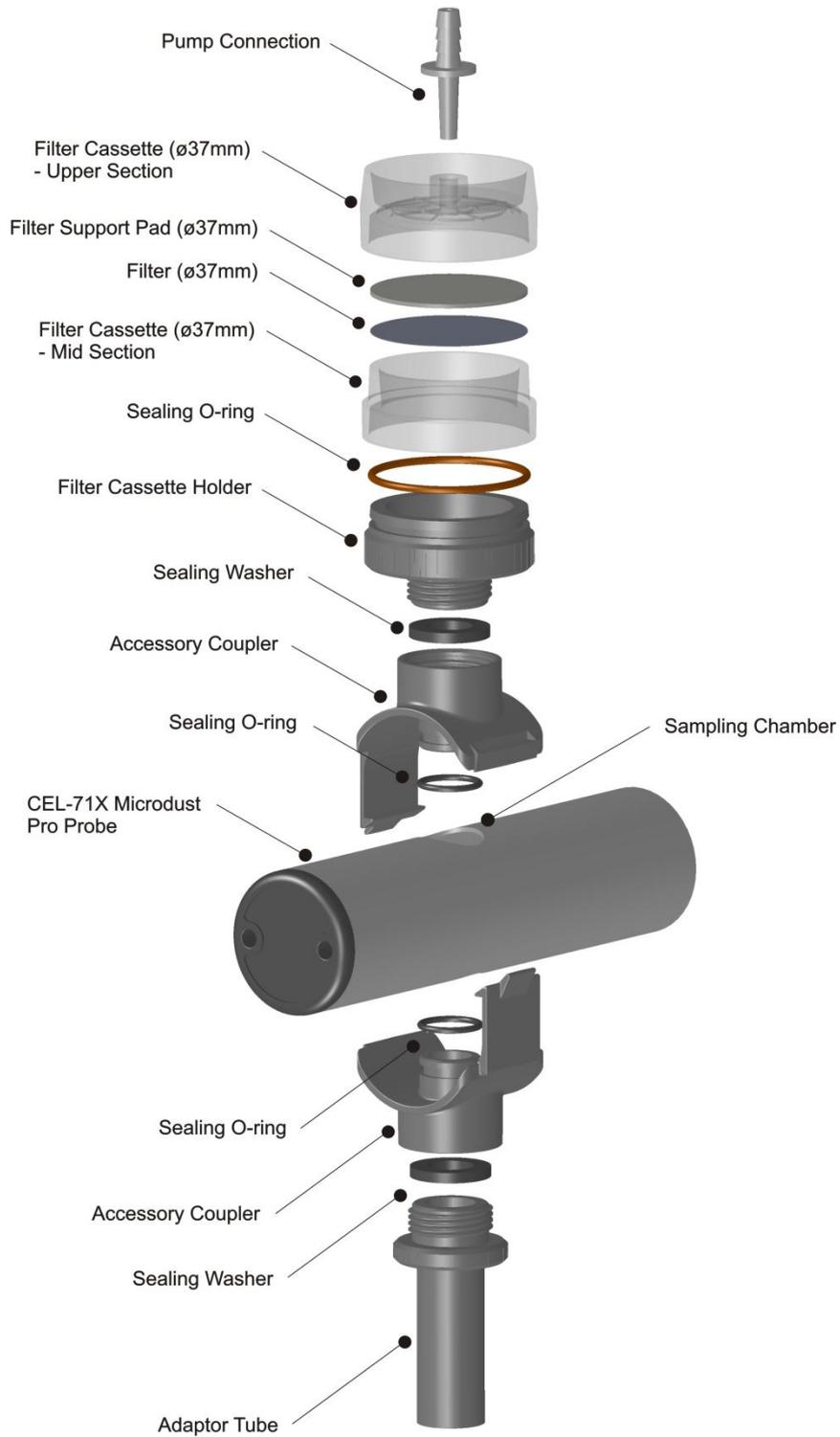
**Figure 24 Microdust Pro Gravimetric Adaptor (Ø37mm Filter)**
