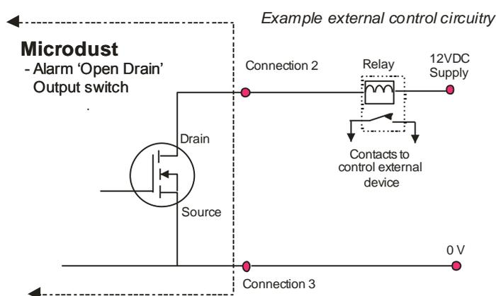
The audible and visual alarm warnings may be cleared by pressing the Accept soft key on the warning screen. The 'Open Drain' output will remain active whilst the alarm condition is valid.
