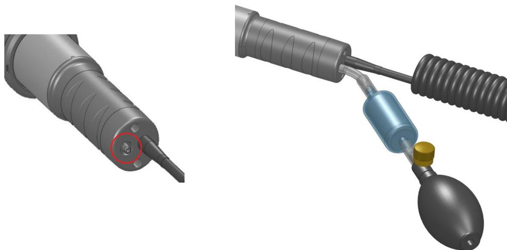
Squeeze and release the purge bellow 5 or 6 times over a 10 second period. This action injects clean air into the chamber and removes possible contamination that might have settled on the optical components inside the probe. When you perform this operation, you might see the indicated concentration increase, and then decrease towards zero.
