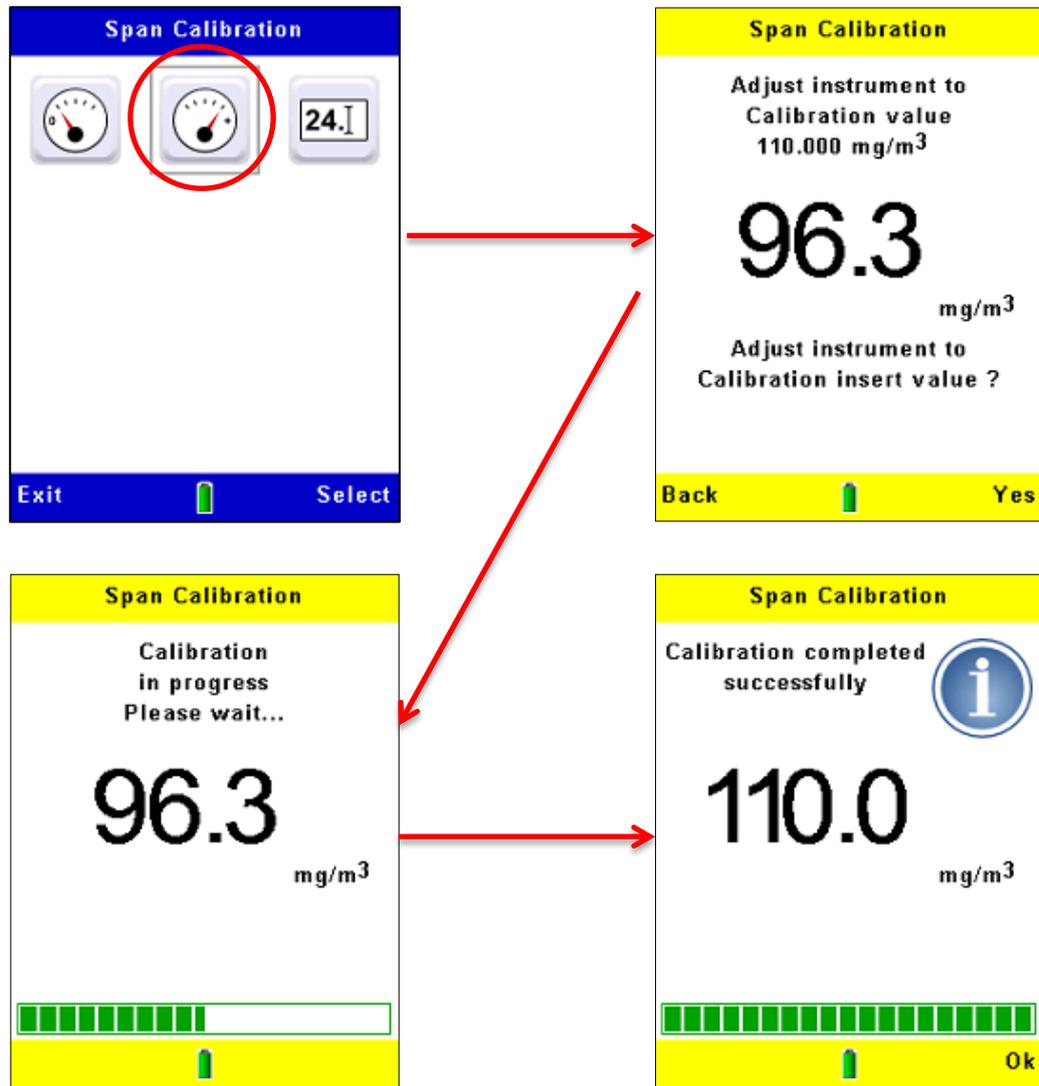
If the correct value is NOT shown (for example because the instrument was last used with a different probe and filter), follow the steps in Figure 17 to set the instrument to use the same reference printed on the Calibration Insert.
