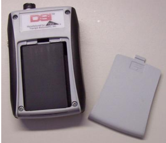
Figure 13 Back of JET device shown with compartment door removed
