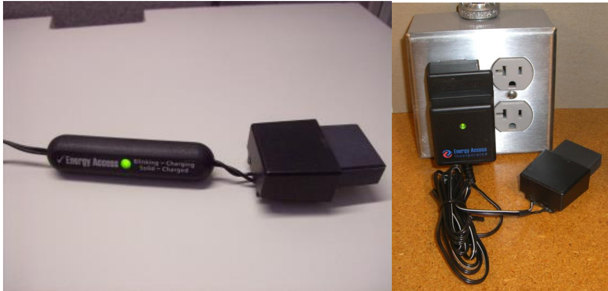
Figure 15 Battery connected to one of the two versions of supplied chargers
