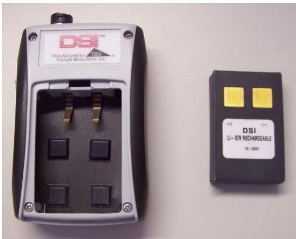
Figure 14 Back of JET device with battery removed
