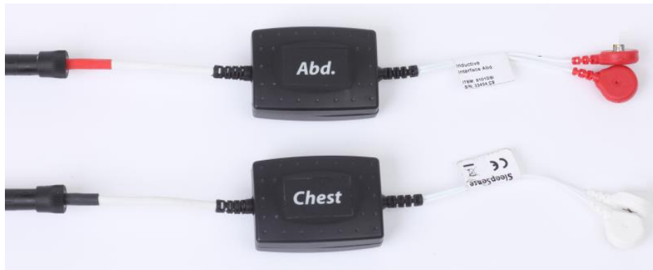
Figure 10 Abdomen and Chest Electronics Modules
