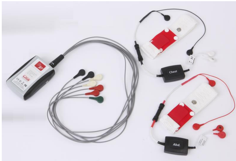
Figure 12 Attachment of Modules to 3 Channel Differential Lead Set
