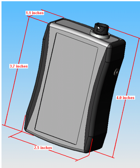
Figure 4 Dimensions of JET Device
