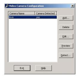
2. The status of each configured camera will update in the **Camera Detected** column of the Video Camera Configuration window.
