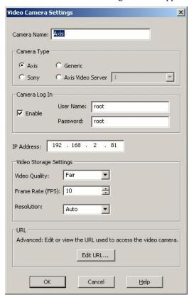
4. Edit the settings in this window then click **OK**. The program will re-verify communication with the camera and return to the Video Camera Configuration window.
