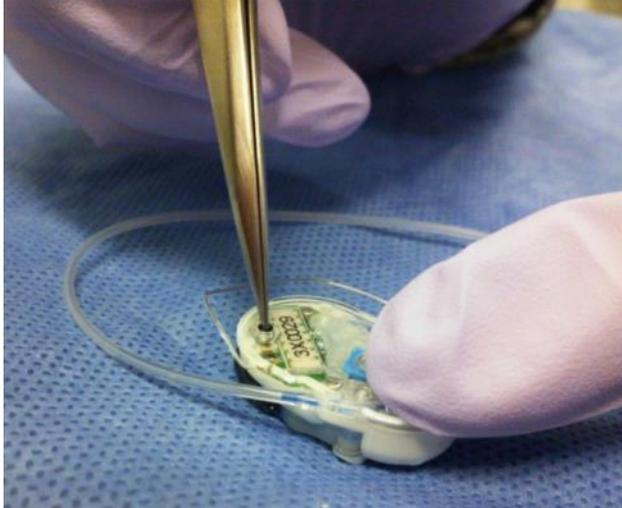
5. When Power On successful, activation starts, and the inner cam rotates for about a 100 seconds where the rear most pin completely blocks the tube. This is for a new un-activated pump. Check by verifying CAM position or that reservoir is locked after 2-3 minutes.
