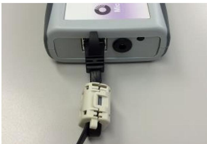
Ferrite core attached end must be connected to UCD-300 side.
