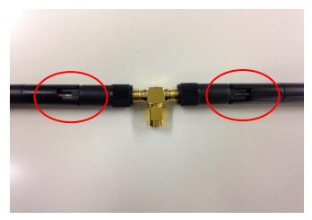
Place the dual antennae onto UCD-300. Hinges are facing upwards to allow antennae to bend upwards.
