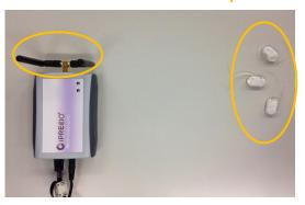
Distance of each antennae to SMP-300 pumps should be different. Above shows best orientation to maximize distance difference.
