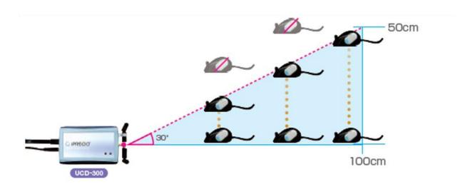
Pumps should placed within 50cm height from the UCD-300 Do not put the pumps lower than the management system.
