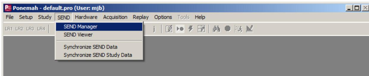
**Figure 14. – SEND Manager access point from the SEND pull-down menu.**
