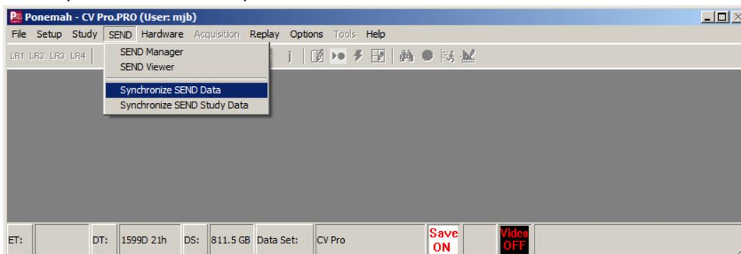
**Figure 27. – Synchronize SEND Data dialog selection from SEND pull-down menu**
