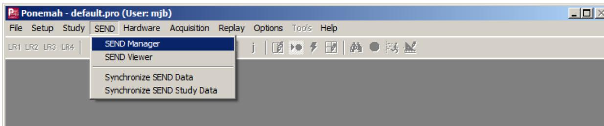
**Figure 14. – SEND Manager access point from the SEND pull-down menu.**
