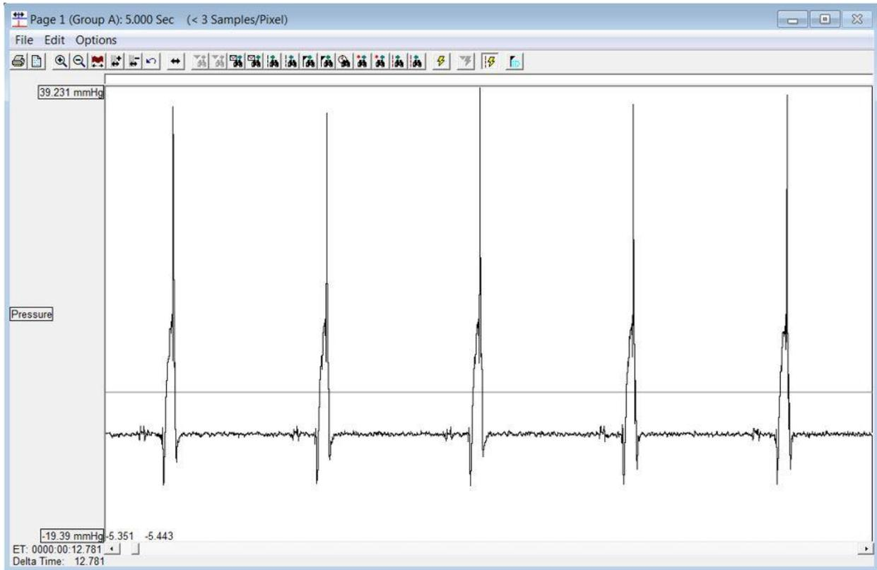
Note: 1 second spikes might be observed on biopotential channels while in the sterile pack or when not yet implanted. These are not from passivation but are an expected result of the high-gain biopotential amplifiers picking up very small voltages from the environment or from the antenna. Once the leads are implanted the biopotential spikes from environmental noise will go away.
