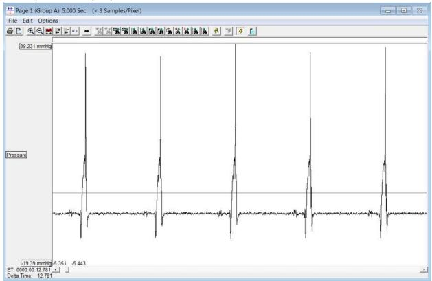
Note: 1 second spikes might be observed on biopotential channels while in the sterile pack or when not yet implanted. These are <u>not</u> from passivation but are an expected result of the high-gain biopotential amplifiers picking up very small voltages from the environment or from the antenna. Once the leads are implanted the biopotential spikes from environmental noise will go away.
