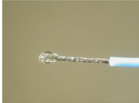
Figure 2: F50-W-F2 Lead/Electrode
