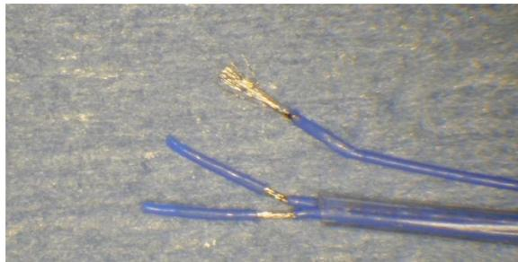
**Figure 16: The Teflon is stripped from the distal portion of the leads to expose the wire and create the electrode to interface to the nerve**
