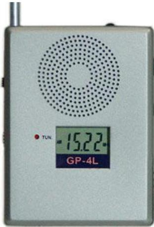
The F50-W-F2 transmits using different frequency (18MHz) than most other DSI transmitters. As a result, a different radio must be used to verify if the transmitter is on or off. The same radio can also be used with a standard DSI transmitter (455KHz). Please refer to the instructions supplied with the GP-4L radio for additional information.
