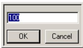
The user can select the units he wishes to display. Combined with Low Cal and High Cal, the user can set the “x” value in Cal to equal the “y” number of Units. Example: If 2.500V is entered in the High Cal and 100 is entered in High Units, then 2.500V = 100 units. See the Measure Section for more information.
