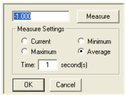
In instances where there is an offset on the input signal, the Measure function can compensate for this offset. The software can Measure a Low or High Cal value, and set that value to equal the entry in the Low or High Units cells.
