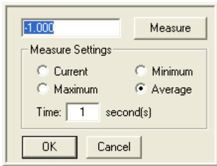
If you have available an input calibration signal (voltage), it can be used to calibrate the inputs. Double-clicking on either the Low Cal or High Cal cell associated with the channel will open a dialog box as shown. This function allows a specific value to be entered that will be assigned to either the Low or High Cal. See the Measure section for more information on this function and the use of the feature.
