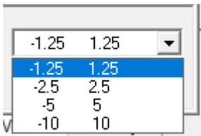
There is one span control that sets the maximum input of the signal conditioner. The span is symmetrical. Ranges available are  $\pm 1.25\text{V}$ ,  $\pm 2.5\text{V}$ ,  $\pm 5\text{V}$ , and  $\pm 10\text{V}$ . The Span defines the sensitivity or scale for each channel. This function sets the maximum and minimum values in user units that will be recorded.
