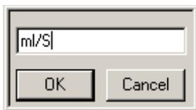
Units allow you to enter the actual engineering units being measured. The default is Volts (V), but this may be changed to any engineering unit. The User Unit input field is limited to 9 characters.
