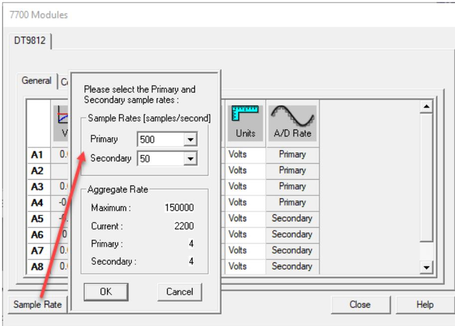
After the Primary and Secondary sample rates are set, each channel can be set to be either Primary or Secondary from the rightmost column called A/D Rate.
