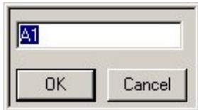
Label allows you to type in a logical name of up to 10 additional characters for a particular input channel. The chosen name will be saved and used to identify the input data throughout the system, such as in the dialog that displays input channel information. The default is the slot letter and channel number in slot.
