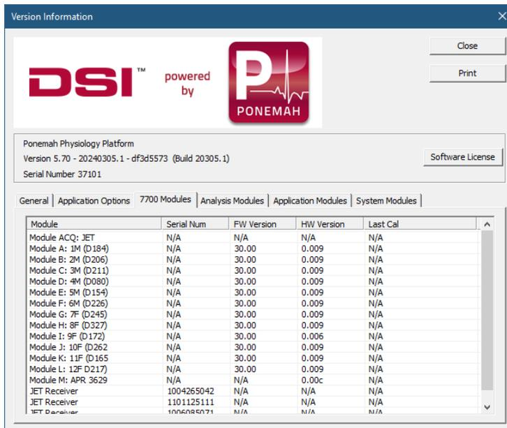
This tab lists each device, the serial number, the firmware and hardware version of each, and the Last Cal Date of each JET device. If the calibration date cannot be stored electronically on the device it will be listed as (NA).
