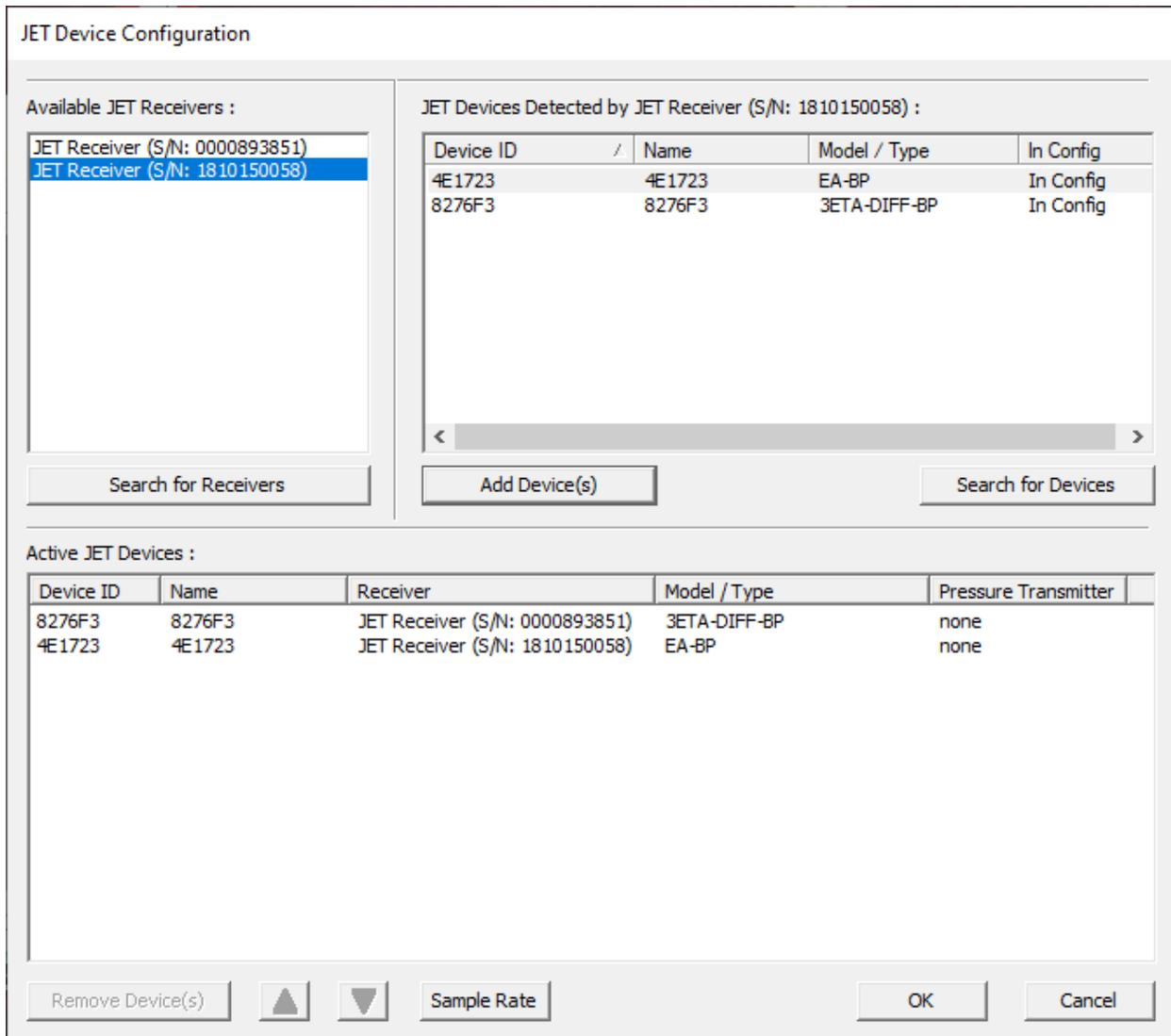
The Active JET Devices section lists the current devices that will be used in the acquisition. The list will include the Device ID, Name, JET Receiver that the device is connected to, and the Model/Type of the device.
