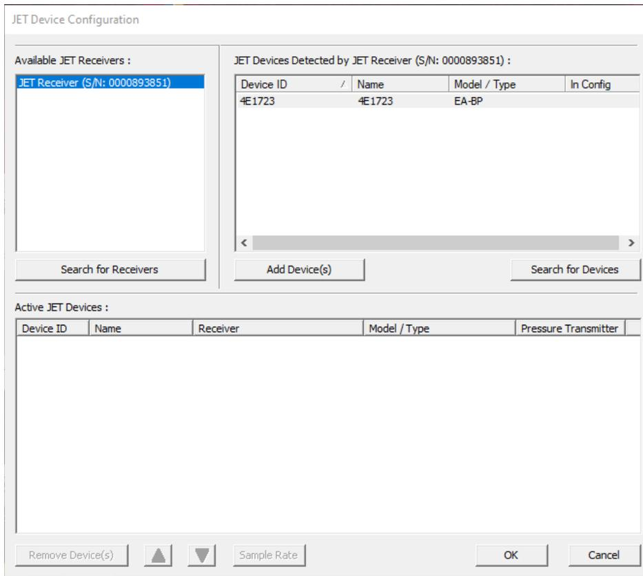
The JET Devices Detected section will list the available devices for the current JET Receiver that is selected. The device that is selected in the JET Receiver section is also listed above the table of information.
