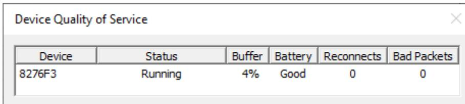
This dialog will show the Device name, Status of the device, the current Buffer size that is being used by the device, Battery state, how often the device needed to reconnect, and how many Bad Packets were sent while acquiring data.
