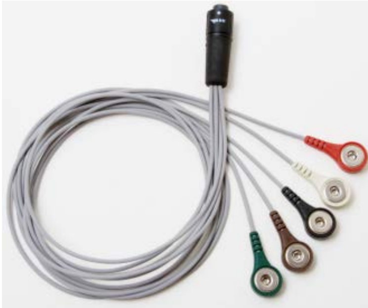
Figure 9 Lead Set for collecting 7 leads of ECG
