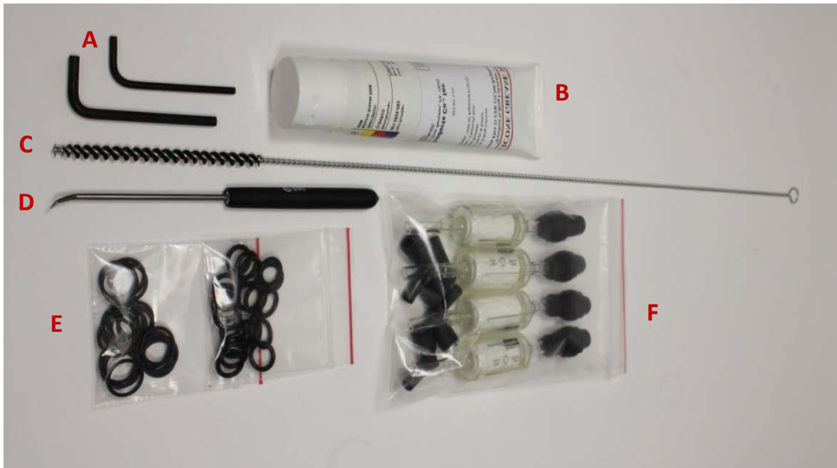
A) Hex keys, B) O-ring grease, C) Bore brush, D) O-ring removal tool, E) O-rings (inner & outer), F) Pump filters
