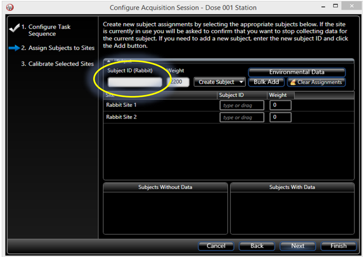
Figure 14. The first page presented when you launch a new data acquisition session. This page allows you to assign subject IDs to each of the site in the hardware configuration.
