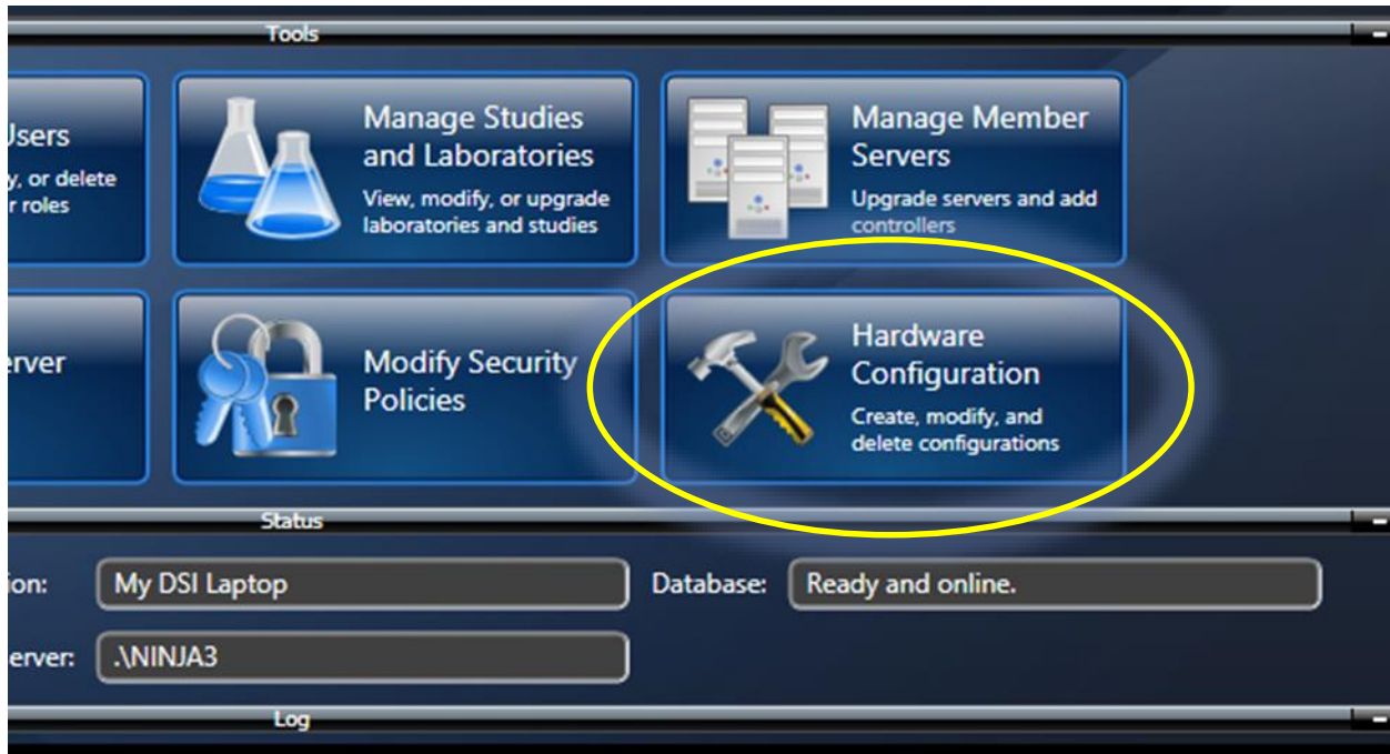
Figure 1. From the main window in the FinePointe Control Panel, click the Hardware Configuration button to create or edit the Dosimetry hardware configuration.
