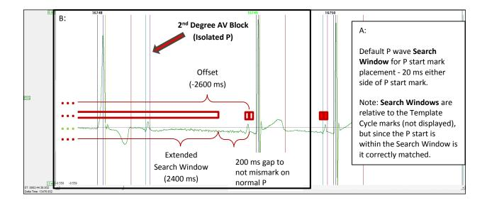
In B, the **Search Window** extends past the data being displayed on the graph. The R wave of the previous cycle acts as a hard cutoff for the **Search Window**. This algorithm has additional logic built in to prevent ECG PRO from marking the T wave of the previous cycle as the isolated P wave.
