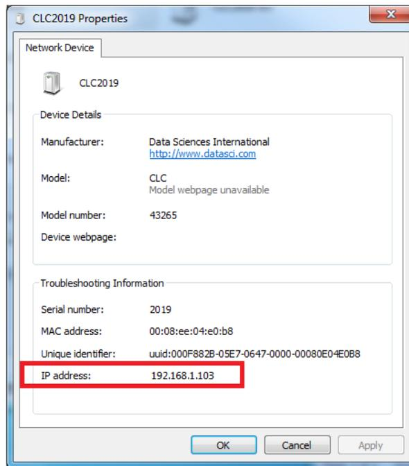
Figure 4 - CLC IP Address in Properties
