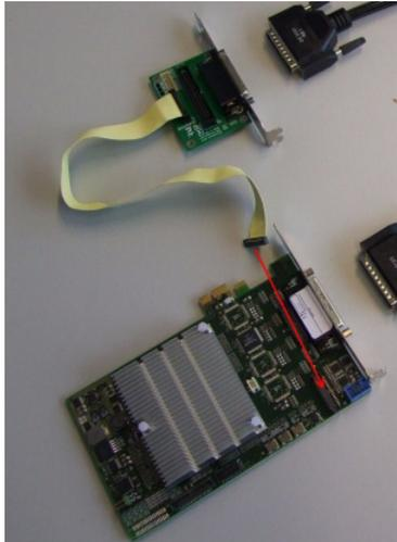
3. Gently but firmly insert the Pico U4, or U8, H.264 encoder card into a free PCI express slot. Avoid touching the contacts or other metal parts of the card.
