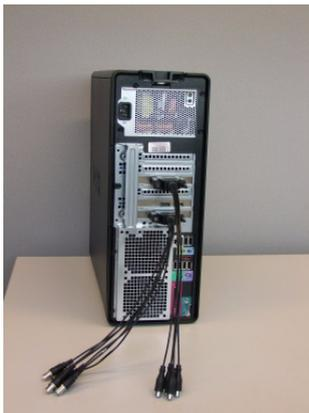
4. Connect at least one video camera to one of the BNC connectors. With the Piccolo U4 H.264 card, do not use the cables with number 5 and 6. With the Piccolo U8 H.264 card, do not use the cables with numbers 9 and 10. When you select the cable labelled with number 1, this is shown as **Euresys Piccolo U4 (or U8) H.264 No/0 - VID 1** in the Media Recorder.
