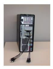
4. Connect at least one video camera to one of the BNC connectors. With the Picolo U4 H.264 card, do not use the cables with number 5 and 6. With the Picolo U8 H.264 card, do not use the cables with numbers 9 and 10. When you select the cable labelled with number 1, this is shown as Euresys Picolo U4 (or U8) H.264 No/o - VID 1 in the Media Recorder.
