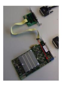
3. Gently but firmly insert the Picolo U4, or U8, H.264 encoder card into a free PCI express slot. Avoid touching the contacts or other metal parts of the card.
