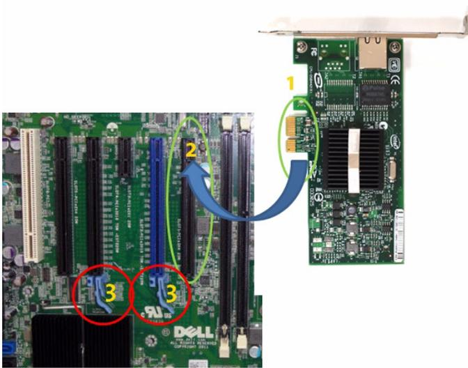
**Figure 2** *Installing the ethernet card into a Dell Precision T3600 workstation. Insert the connector of the card (1) into the slot (2). Do not use one of the slots with a blue hook (3), since these are graphics slots.*
