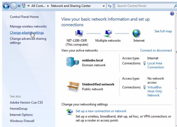
3. Right-click the **Local Area Connection** and click **Properties**. If your computer has more than one Local Area Connection, choose the one to which you are going to connect your IP camera. To check which one this is, remove the cable from this IP port on your computer. The LAN connection that gets a red cross through it, is the correct one.
