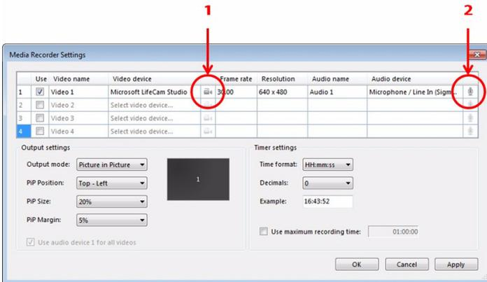
**Figure 1** The Settings window of Media Recorder, with the buttons for the advanced video settings (1) and the advanced audio settings (2).
