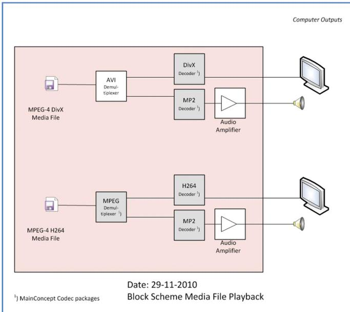
**Figure 6** *Decoding the video files created with Media Recorder.*
