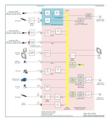
Figure 5 Conversion of video and audio streams by Media Recorder.
