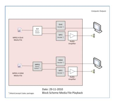
**Figure 6** Decoding the video files created with Media Recorder.
