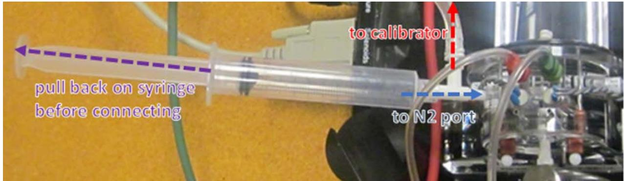
You will need this so that you can push air into the manifold and the calibrator simultaneously.
