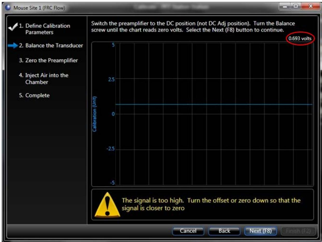
Any warnings are indicated below the chart as shown in the following screenshot. In this example, the instructions say you must turn the Balance screw until the voltage is at zero. FinePointe checked and the signal is too high (it is 0.693V). Click **Next**.
