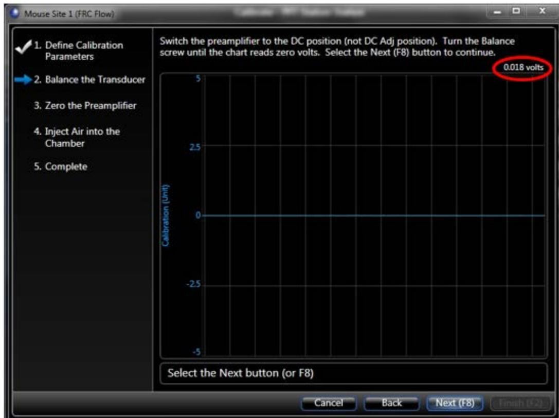
The calibration wizard begins at step 2 “Balance the Transducer”. As with all wizards in FinePointe software, the list at the left shows you the steps you will need to complete in order to finish the wizard, indicating which step you are on by the blue arrow. The scrolling chart on the right shows you the current live waveform. The text above the chart describes what you need to do during this step.
