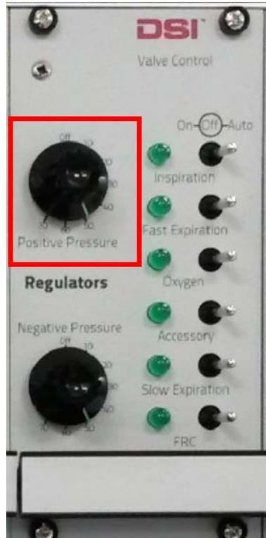
Use the 8-position knob labelled **Positive Pressure** on the Valve Control module to set the desired pressure level. For most situations, set this to 50.
