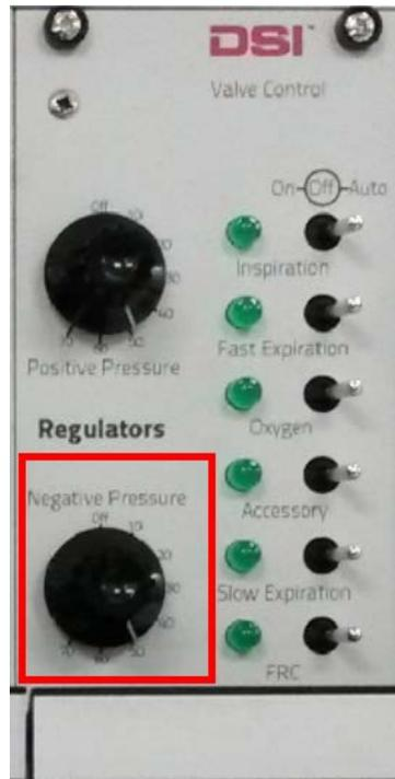
Use the 8-position knob labelled **Negative Pressure** on the Valve Control module to set the desired pressure level. For most situations, set this to 50.
