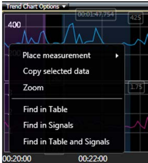
Figure 122. Displays the right-click menu options of a selected section of data from the Trend Charts.
