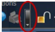
Figure 88. This signifies a sub-command menu. When you click on it, it will reveal additional command buttons.
