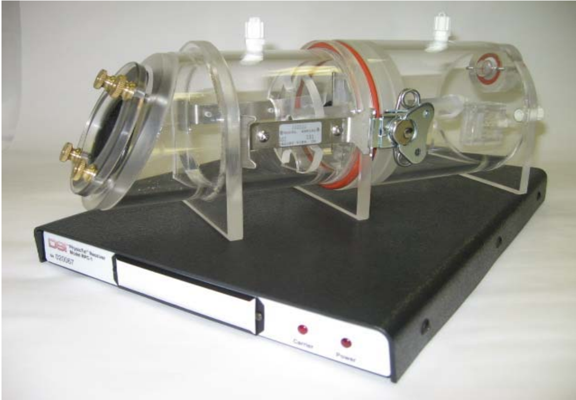
Rat Head-Out Plethysmograph Chamber (600-2100-001) pictured on a telemetry RPC1 receiver plate
