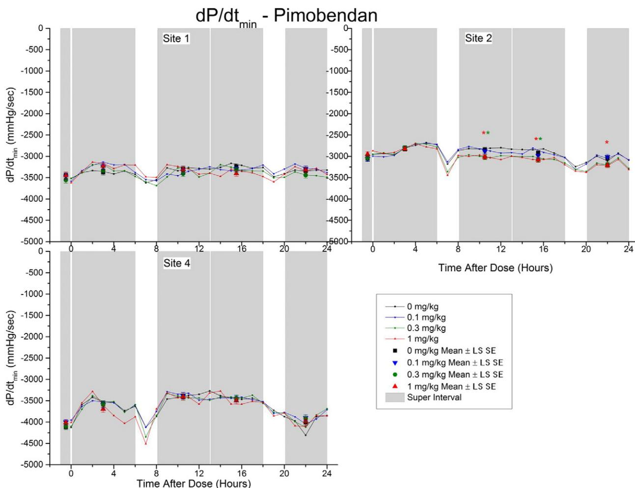
**Fig. 12.** The effect of pimobendan on LV  $dP/dt_{\min}$  in conscious instrumented dogs at three different laboratories (sites 1, 2 and 4). Pimobendan (vehicle =  $\square$ , 0.1 mg/kg =  $\nabla$ , 0.3 mg/kg =  $\bullet$ , 1 mg/kg =  $\Delta$ ) was administered orally at time = 0. Small symbols represent the mean value from the previous 10-min while shaded areas represent super-intervals as defined in Table 3. Large symbols represent the mean  $\pm$  SE within each super-interval.
