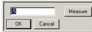
In instances where there is offset on the input signal, the Measure function can compensate for this offset. The software can Measure a Low or High Cal value, and set that value to equal the entry in the Low or High Units cells.
