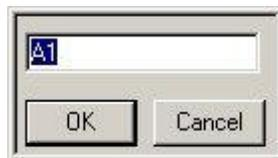
Label allows you to type in a logical name of up to 10 additional characters for a particular input channel. The chosen name will be saved and used to identify the input data throughout the system, such as in the dialog that displays input channel information. The default is the slot letter and channel number in slot.
