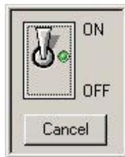
The State function will turn the sampling on or off for that channel, but the last value will continue to be displayed. It is recommended that this selection should always be left in the ON condition. To turn any channel on or off, set the analysis to DIS in the P3 Setup dialog. The default is ON.
