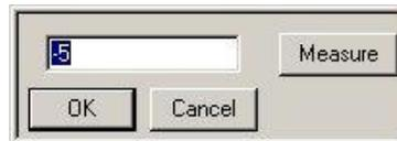
If you have available an input calibration signal (voltage), it can be used to calibrate the inputs. Double clicking on either the Low Cal or High Cal cell associated with the channel will open a dialog box as shown. This function allows a specific value to be entered that will be assigned to either the Low or High Cal. See Measure section for more information on this function and the use of the feature.
