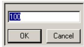
The user can select the units he wishes to display. Combined with Low Cal and High Cal, the user can set “x” value in Cal to equal “y” number of Units. Example: If 2.500V is entered in the High Cal and 100 was entered in High Units, then 2.500 V = 100 units. Also see Measure Function.
