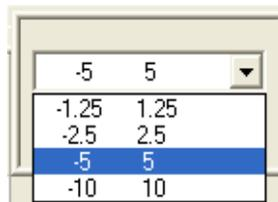
There is one span control that sets the maximum input of the signal conditioner. The span is symmetrical. Ranges available are  $\pm 1.25\text{V}$ ,  $\pm 2.5\text{V}$ ,  $\pm 5\text{V}$ , and  $\pm 10\text{V}$ . The Span defines the sensitivity or scale for each channel. This function sets the maximum and minimum values in user units that will be recorded.
